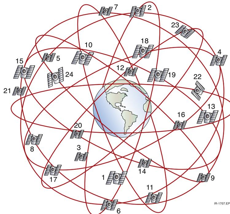
**Figure 1-3** The orbital configuration of the 21 GPS satellites.
