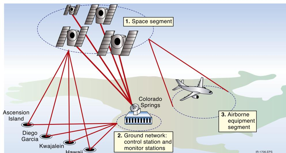
Figure 1-2 The GPS consists of three basic segments.
