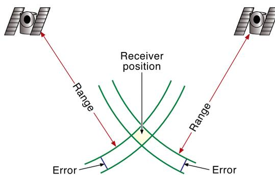
Figure 1-7 Good satellite geometry resulting in low PDOP.
