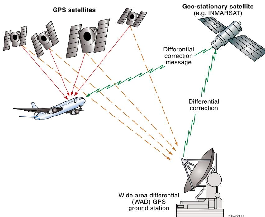
**Figure 1-10** Concept of wide area differential GPS.
