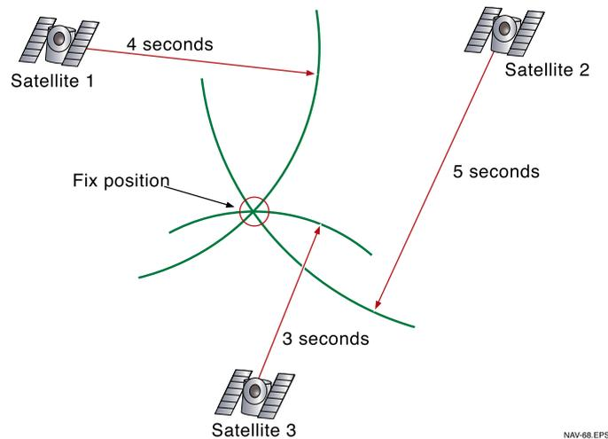
**Figure 1-4** Two-dimensional fix established with perfect timing.
