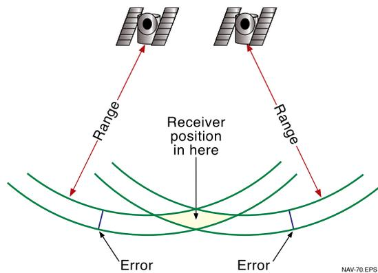
Figure 1-6 Poor satellite geometry resulting in high PDOP.
