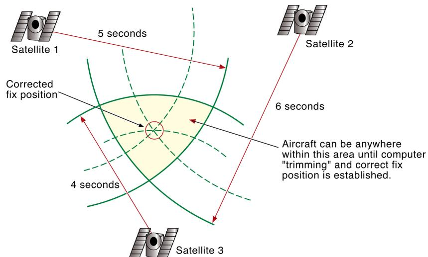
**Figure 1-5** Effect of receiver clock error of 1 second on two-dimensional fix.
