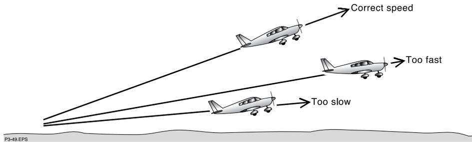
Figure 3-8 Fly at the correct speed for the best performance.
