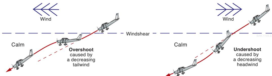
**Figure 7-20** Effect of windshear in the descent.
