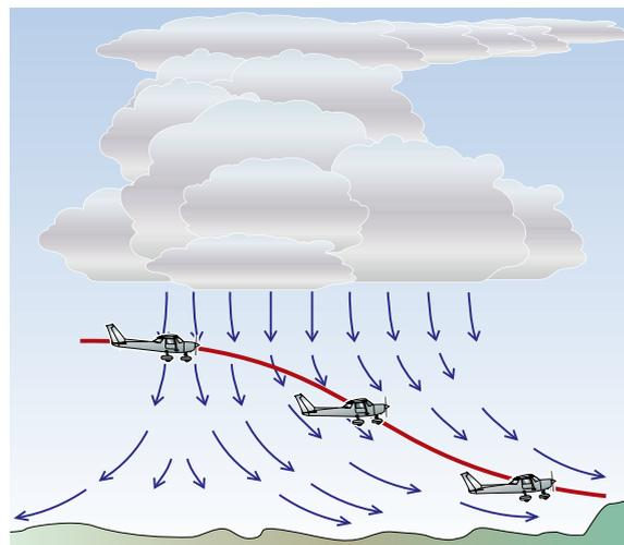
**Figure 18-13** Severe downdraughts beneath cumulonimbus (Cb) storm cloud.
