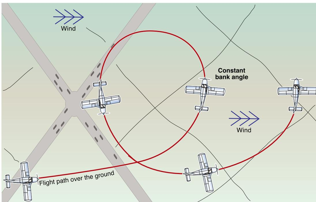
**Figure 18-9** Aircraft path relative to the ground
