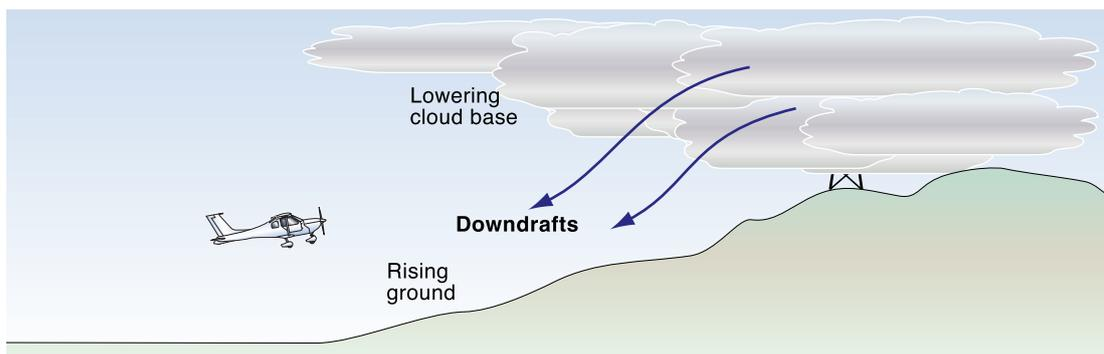
**Figure 18-11** Be careful of rising ground, lowering cloud and downdrafts
