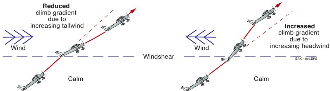
**Figure 18-10** Effect of windshear in the climb.
