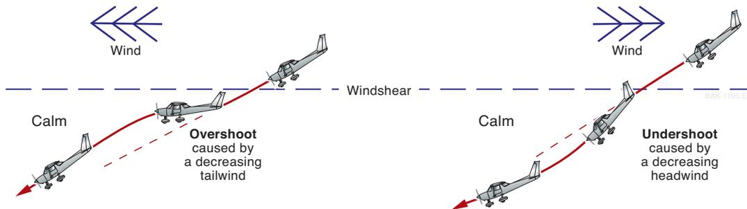
**Figure 18-12** Effect of windshear in the descent.
