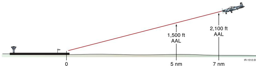
**Figure 7-9** A 3° glideslope loses height by about 300 ft/nm.
