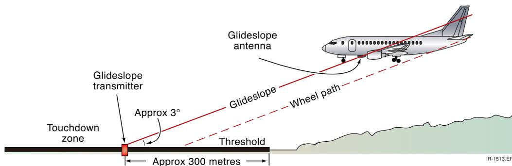
**Figure 7-10** The typical glideslope transmitting antenna is approximately 1,000 ft in from the runway threshold.
